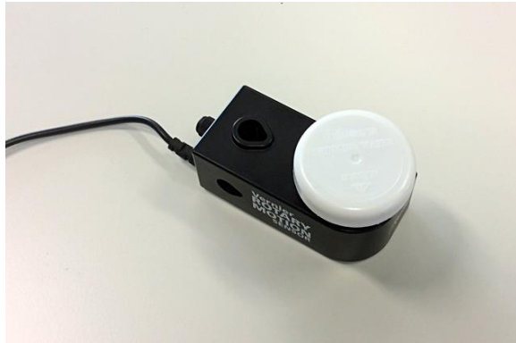
Fig 1 – a Vernier angular motion detector with a plastic disc attached.
