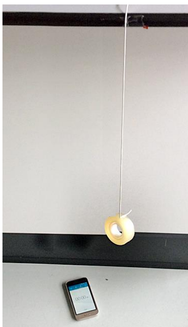
Fig 1 – a simple pendulum and a telephone-based stopwatch.
