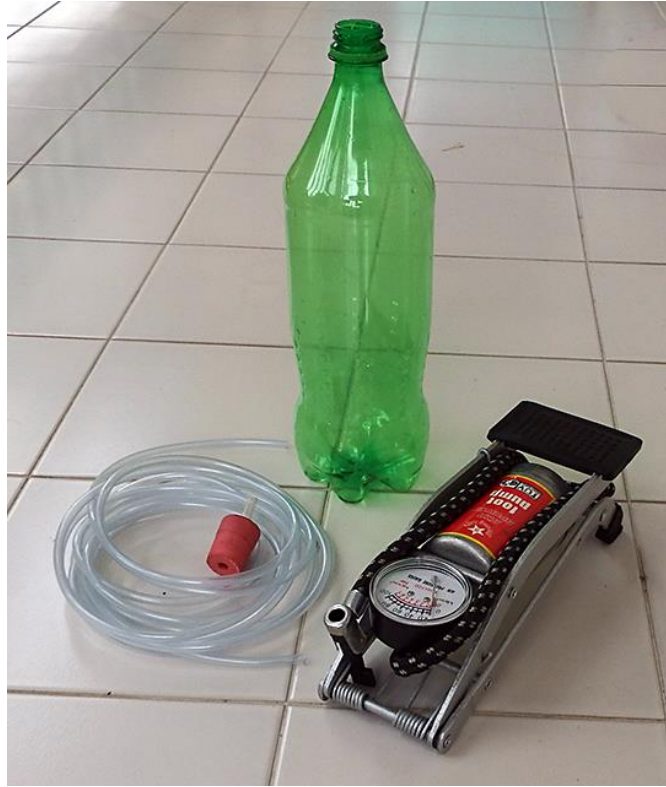
Fig 4 – equipment for making a cloud in a bottle.
