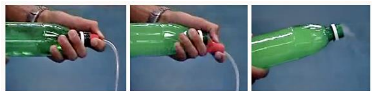
Fig 5 – Cold air rushes out and a cloud appears in the bottle.
