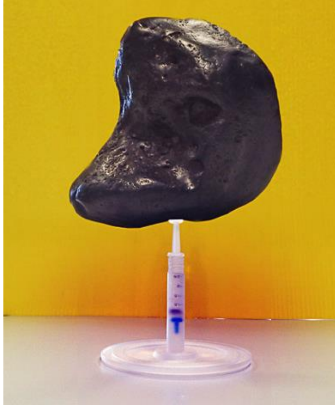
Fig 1 - 55 newtons rest on a syringe. The weight is supported by the compressed air in the small space above the blue clay plug.
