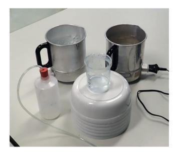
1 The bottle (in one hand) is placed in the hot water at  $\sim 90^{\circ}$ C (in the pot on the right). The pressure rises and a little water is lifted in the hose (held in the other hand) to fall from 20 cm above the beaker.
