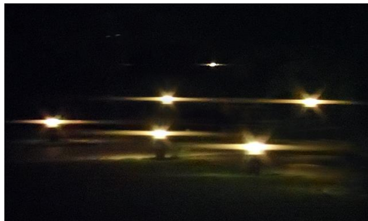
Fig 6 – diffraction produced when a vertical 0.5 mm slit was placed in front of the camera lens.
