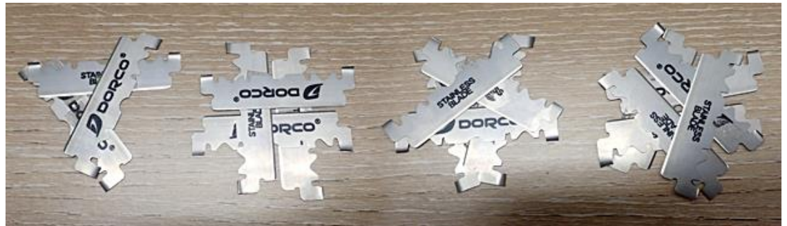
Fig 3 – apertures constructed with razor blades.
