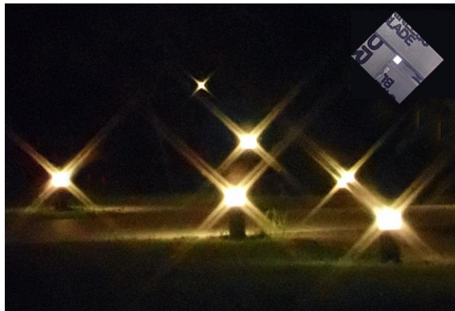
Fig 2 – diffraction points surround lights at night in this digital camera image taken with a square aperture placed in front of the lens (inset).
