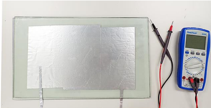
Fig 4 – the capacitor reassembled with just half the original area of overlap.
