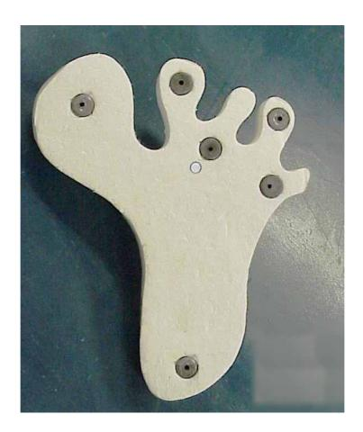
A good approximation to the centre of mass (that lies inside the small circle) can be found by defining axes, measuring and calculating as above. If a correction for the mass of the polystyrene is required the centre of mass of the irregular sheet is best found by removing the lead, hanging from different points and drawing verticals, or by finding the point of balance when horizontal, or by finding the rotation axis about which no vibration occurs.
