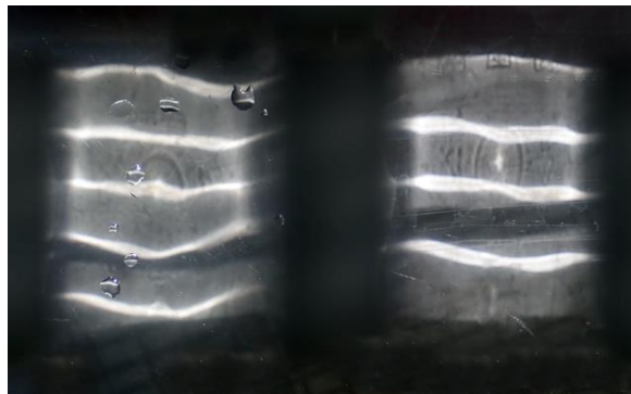
Fig 9 –at slightly higher frequency with wavelengths close to 3 cm.
