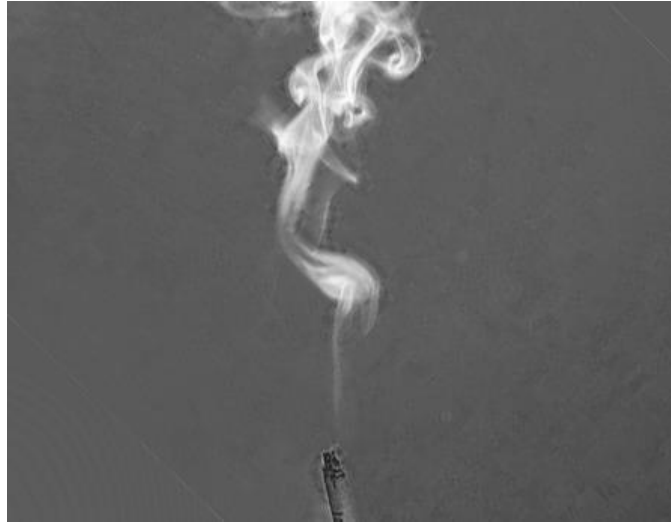
Fig 1 – cigarette smoke transitions from laminar to turbulent flow.
