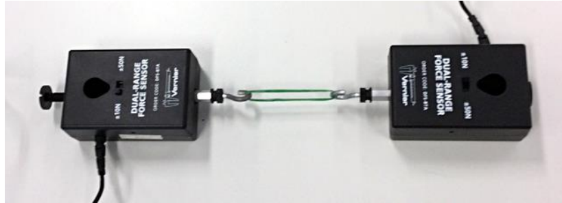
Fig 7 – a calibrated force-probe (left) linked to a second probe.
