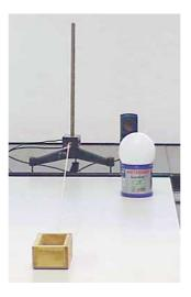
In the new design the force probe is attached to a clamp stand on a fixed bench behind the table. The table is on castors \*wheels" and is pulled away from the bench. A motion detector on the bench records the position of a ball, fixed to the table, as a function of time to make a force-velocity plot.
