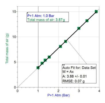
Pressure is proportional to the mass of air in the bottle and the density of air is confirmed as ~1.3 kg per m<sup>3</sup>, accurate enough for demonstration purposes.
