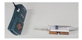
Note: a low-friction glass syringe could be used for this demonstration but a cheap plastic syringe is satisfactory. A 5 or 10 ml narrow-barreled syringe allows the plunger to be moved by hand without excessive force.
