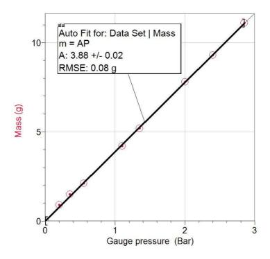
Extending the straight line to an origin at zero pressure converts gauge pressure to absolute pressure.
