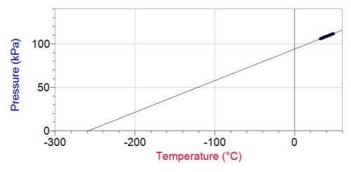
The intercept suggests an absolute zero of temperature at about -260 °C. Pressure is then proportional to the absolute temperature. An extrapolation of this extent is not normally justified but this initial estimate of absolute zero is close to the known value of -273 °C. It is important when doing this demonstration to eliminate leaks from the bottle. Failure to do so results in a false estimate of absolute zero that is much closer to 0°C.
