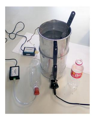
A PET bottle filled with air is connected to a pressure sensor and submerged in water in an extended pot. The water is warmed and constantly stirred.
