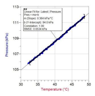
As the temperature rises the pressure/temperature plot is a straight line.
