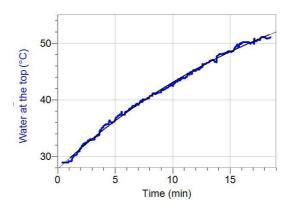
The rise in temperature near the top of the water column is exponential as shown by the curve fit. Almost all heating curves without a change of state have this form.
