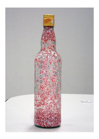
When the bottle is gently heated at the base with warm hands the flow is turbulent. Text-book diagrams of convection with laminar flow owe more to imagination than observation. If a class enters a cold room and sits close to the bottle slow convection currents are driven by radiated body heat.
