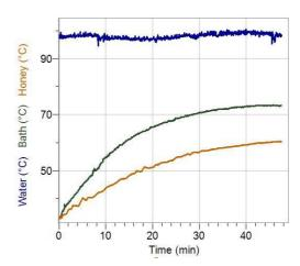
Temperature rise with time is shown in the tops of the bottles when the water bath was held at 95°C.
