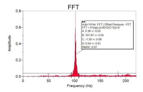
**a** The resonance frequency has been found by fitting a Gaussian function to the FFT plot. How could the frequency be found from a data plot in the time domain?
