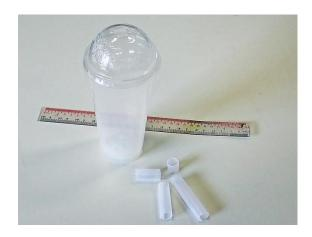
The round hole in the cap has a diameter of 1.45 cm. Short lengths of plastic pipe with an internal radius of 0.65 cm convert the container into a Helmholtz resonator. Measured resonant frequencies are plotted below against frequencies calculated with the Helmholtz relationship  $f = v/2\pi \left[A_x/VL\right]^{1/2}$  for four pipe lengths.
