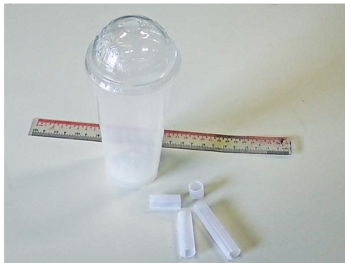
Fig 2 - the components of a demonstration Helmholtz resonator.
