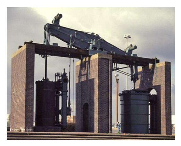
This original Boulton-Watt engine was as big as a three-story house and delivered about 30 horsepower. It has been rebuilt as a monument on a road near Birmingham. There is just one Boulton-Watt engine in England (from 1812) that still works. https://en.wikipedia.org/wiki/Crofton Pumping Station#Description
