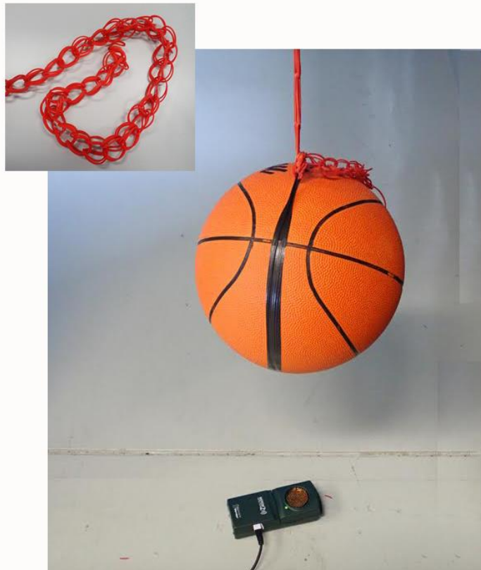
Fig 1 – a basketball hangs from a force probe (not shown) on a rubber-band bungee above a motion detector.
