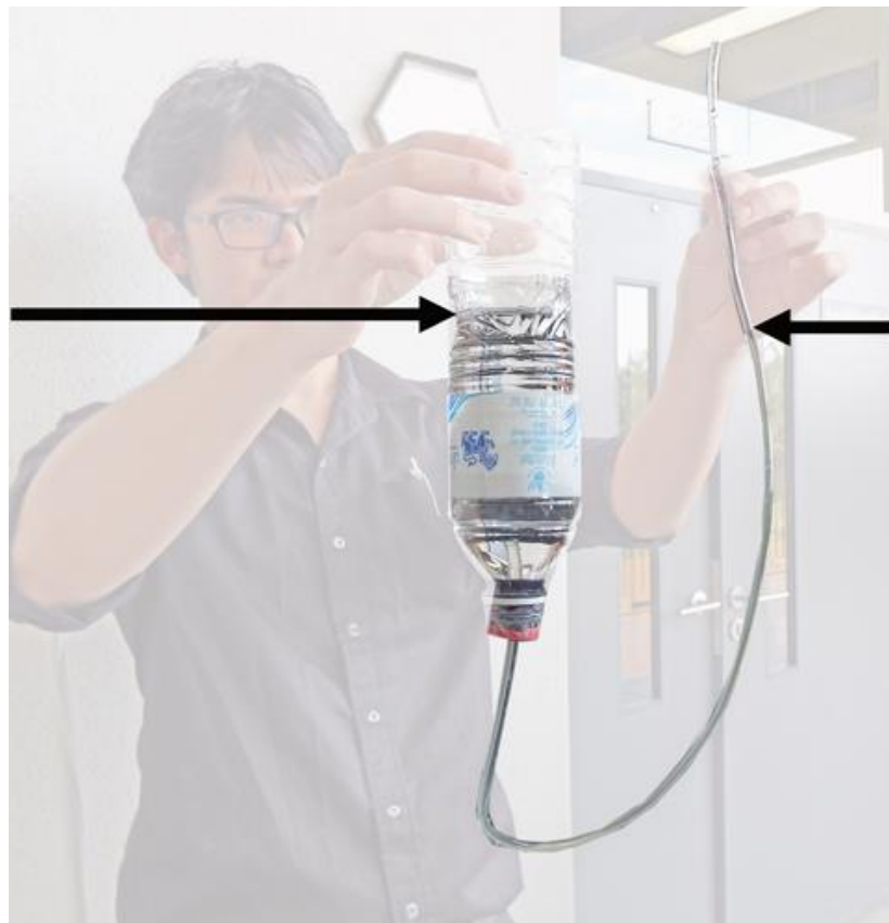
Fig 1 – an unequal arm water manometer open to the atmosphere.
