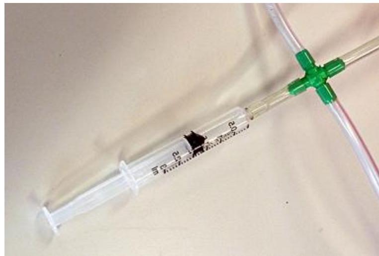
Fig 1 – syringe and connections to two manometers and a pressure probe.
