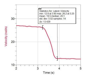
The moment of inertia was found by calculation to increase from 0.0012 to 0.0023 kg  $m^2$ .
