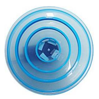
The plate is set spinning. Three 30 gram masses are dropped at the same time by hand into the outer ring. The angular velocity of the plate reduces.
