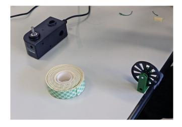
The pulley and motion detector are mounted so that a string is horizontal and winds naturally onto a spool that has a radius of 1.45 cm.
