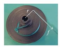
A plastic plate with rings as shown is fixed to the spool which is then mounted on the angular motion detector.
