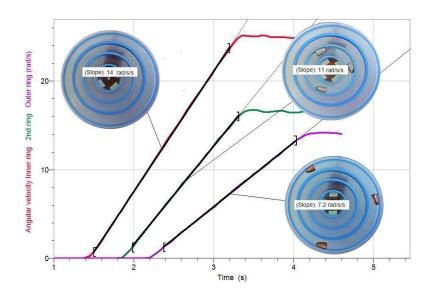
The figure has been prepared by pasting data columns copied from individual Logger Pro files to *New Manual Columns*. Moments of inertia  $I = I_0 + I_{3m}$  can be found from equation 3 using the known torque fr and the measured angular acceleration  $\alpha$ .
