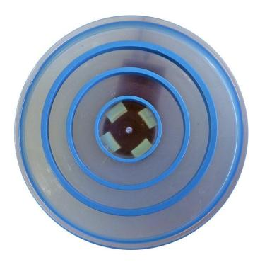
A falling weight on the end of the string applies a constant torque  $\mathit{fr}$  to the plate. The acceleration of the plate  $\alpha$  is the slope of the angular-velocity/time graph in radians/s/s. From equation 2, the moment of inertia of the plate and rings is given by ...
