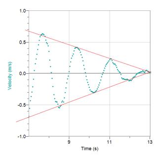
Lines have been added in red to show the almost identical reduction in velocity each cycle.
