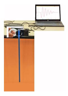
The damping torque is constant and the amplitude decays by close to the same amount each cycle.
