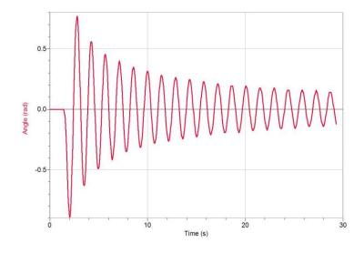
Removing the ball and pressing a smooth reel of tape gently against the rotating disc replaces the damping force in air with a near constant torque to oppose the motion.
