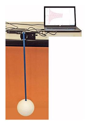
The dominant damping force is due to turbulence in air. The amplitude decays as shown below.
