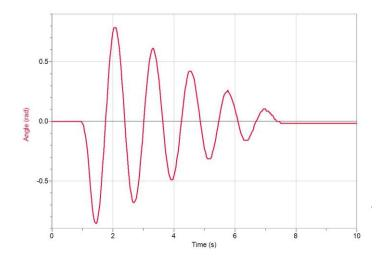
At small amplitudes and near constant angular frequency, maximum velocity is equal (for SHM) to  $A\omega$  and the velocity again reduces by almost the same amount each cycle.
