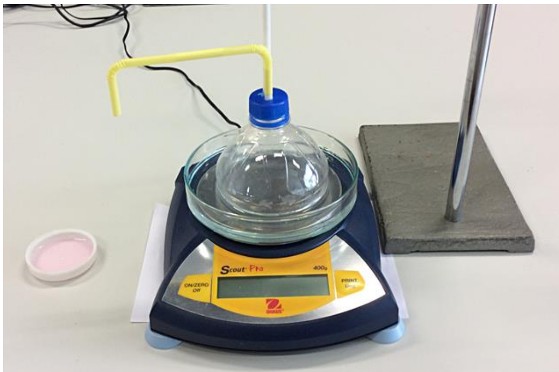
Fig 2 – improvised apparatus for measuring soap bubble gauge pressure.
