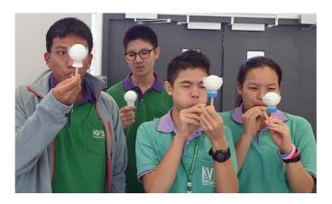
The balls *cannot* be blown out of the cups because fast moving air lowers air pressure on the lower surface. Turning the cups over allows the balls to be held in place by blowing through the straw. The force due to the Bernoulli effect can be measured with a force probe.
