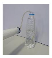
Swinging one metre of pipe at eight radians per second raises the water in the aquarium hose by about 30 mm indicating that the motion lowers the pressure in the closed pipe by about 300 Pa. Holding the open end of the pipe at right angles out the window of a car driven at 8 m/s raises the water in the aquarium hose by 4-5 mm (40-50 Pa) due to the Bernoulli effect. The pipe in the moving car remains silent when the inner end is opened.
