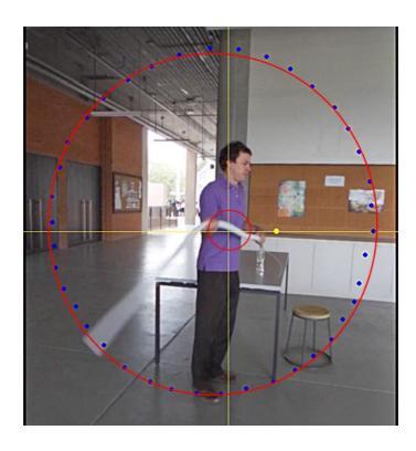
Data points on the outer circle show the tube position at intervals of one thirtieth of a second. It is tempting to say that airflow outwards through the pipe is due to a lowering of pressure at the outer end because air is passing over the open end of the pipe with velocity  $\nu$  (Bernoulli's principle).
