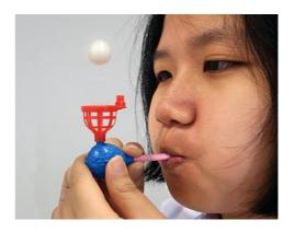
The ball can be lifted upwards from the basket by blowing, but not from a cup.
