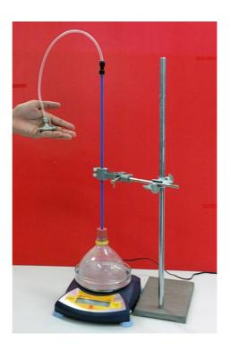
The flow is turbulent but an estimate of airflow velocity can be made from the weight reduction and the area of water inside the chamber.
