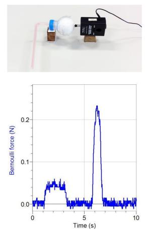
'Emptying' the lungs over 2.0 seconds when the gap between the ball and the bottle is  $\sim 5$  mm gives a small force of 0.05 N. Emptying the lungs in half the time (1.0 s) increases the force by about four times as expected.
