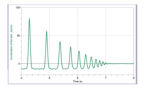
Subtracting the constant acceleration due to gravity and calculating the force as f = ma with a measured mass of 61 grams for the ball gives the graph below that shows the force on the floor as the ball bounces several times and then comes to rest.
