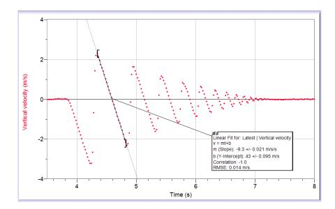
If we can neglect air resistance the acceleration of the ball will be constant when the ball is clear of the floor. Velocity-time lines on the lower graph will be straight (as shown) with a slope close to the acceleration due to gravity, -9.8 m/s/s.
