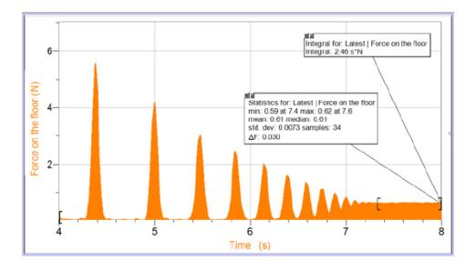
Dividing the integral in Ns by the time (4 seconds) gives (within errors) the average force on the floor as the weight of the ball. (2.46/4.0 = 0.61 N).
