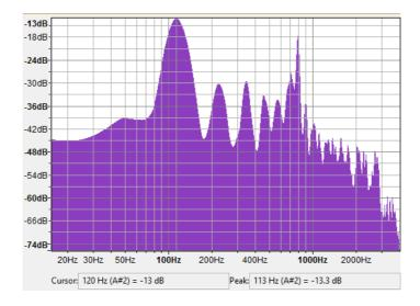
The frequency of the lowest (dominant) mode with one half wavelength on the rubber band is given in audacity as 113 Hz. The tension T in the rubber is given by the force probe reading as 5.48 N. The measured length L to the nearest mm is 41.8 cm.
