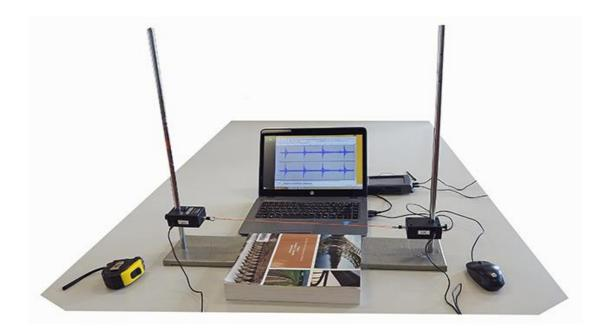
The rubber is repeatedly plucked and the sound is recorded in Audacity.
