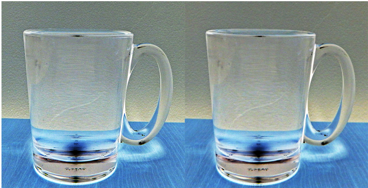
Fig 1 – The cup is full to the brim at 100^{\circ}\text{C} (left) and not so full at 20^{\circ}\text{C} (right).
