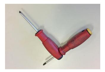
The hole is for inserting another screwdriver so more torque to be applied by hand, and greatly increased torque broke the blade.
