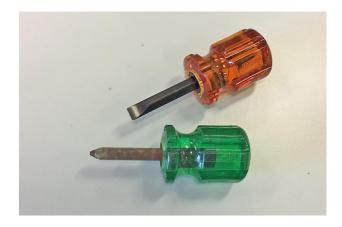
The screw driver below has a hole in the handle and the blade is broken.
