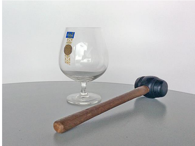
Fig 5 – wine glass with added mass (one baht coin).
