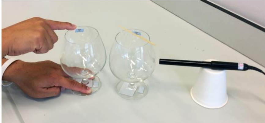
Fig 7 – the right hand glass rings in response to the ringing tones of the left hand glass.
