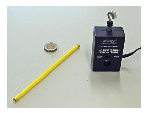
Holding the tube vertically at a measured distance above the probe (to keep the radius of the circular motion constant) and rotating the mass at different high speeds plots a tension versus time graph modulated by the frequency of rotation.
