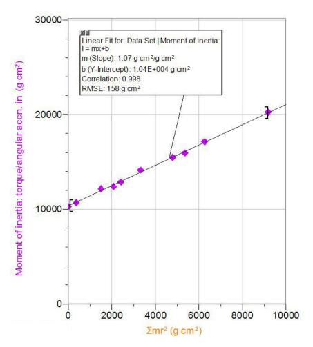
A straight line has been fitted to the data points. The intercept on the vertical axis is the moment of inertia of the empty plate. The close linear fit with a slope close to one shows that the moment of inertia for the small 30 g masses is proportional to the radius squared as expected. Why might the slope differ slightly from the expected value?
